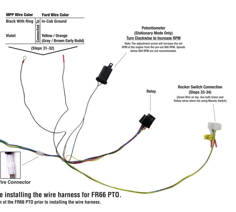
**20.** Separate the wire harness at the 6-Wire connector. The engine compartment portion of the wire harness has (7) connections: the
